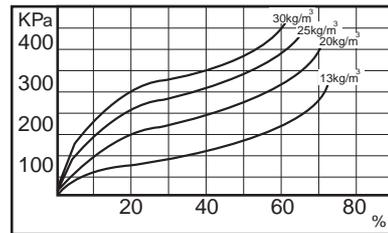
Fig. 5: Stress v compressive strain
