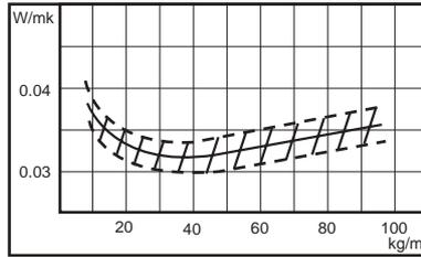
Fig. 7: Thermal conductivity at 10°C v density
