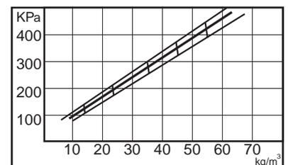
Fig. 4: Shear strength v density at 23°C
