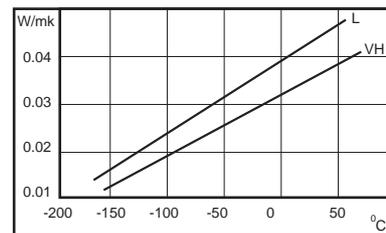
Fig. 9: Indicative thermal conductivity v temperature
