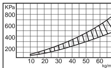
Fig. 1: Stress at 10% deformation v density
